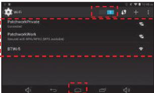
4) Enable Wi-Fi. Choose the name of the hotspot and enter the access code. Once connected press **Home** and then **Start BlackBox Air**.
