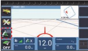
1) When in the job screen with the Field Boundary loaded, press **Guidance Options**.
