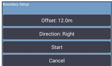
3) Press **Start** and drive around the field edge until the start point is reached. The BlackBox will automatically close and save the boundary map, displaying the field shape and area size in the mini map. If the boundary doesn't close, press the **Close Boundary** button.
