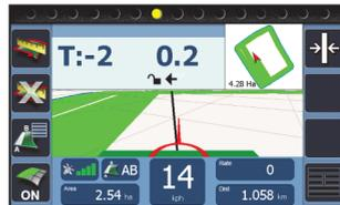
Pressing the **Grid area** a third time allows the guidance line to be reset and also if using the 'Straight' guidance mode, recalibrated to align with current location.
